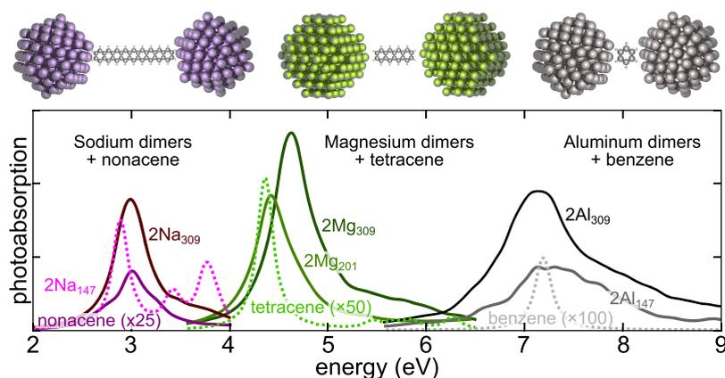
**Figure 1.** Schematic illustration and photoabsorption spectra of the studied nanoparticle-dimer systems spanning a broad spectral range from visible to UV. From left to right: sodium dimers with 30 Å gap (resonance at 3.0 eV) with nonacene (electronic transition of  $\mu = 15.3$  D at 2.9 eV), magnesium dimers with 18 Å gap (4.6 eV) with tetracene (11.1 D, 4.4 eV), and aluminum dimers with 10 Å gap (7.2 eV) with benzene (4.4 D, 7.2 eV).
