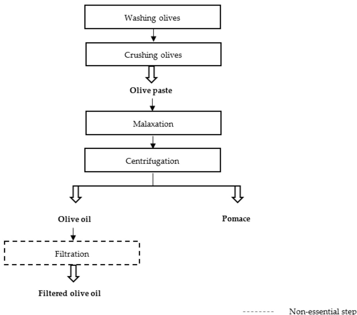
**Figure 1.** The continuous extraction process of olive oil.
