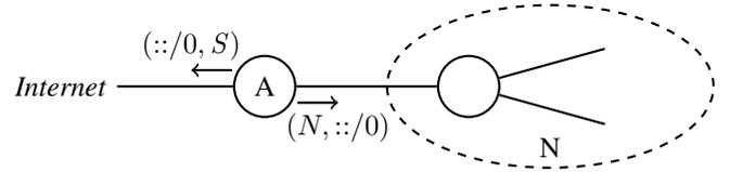
Fig. 3. A stub network behind a source-specific router
